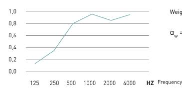
Weighted sound absorption coefficient:
